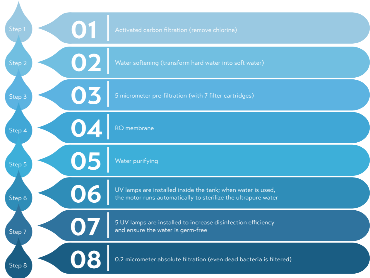
● Figure2-14 Eight-step ultrapure water manufacturing process
